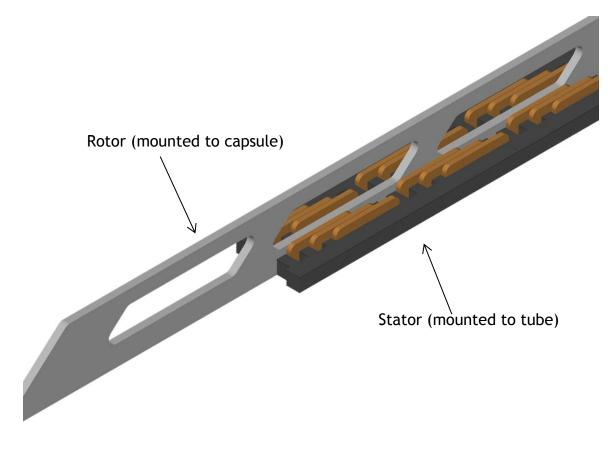
Figure 21. Rotor and stator 3D diagram
