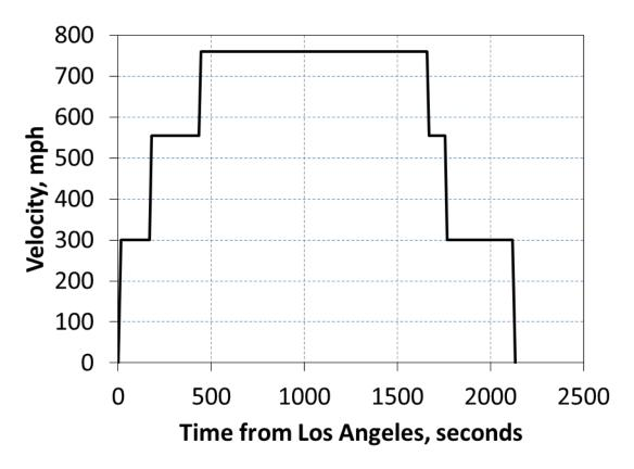
Figure 26. Velocity of capsule as a function of time from Los Angeles departure.
