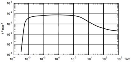
Figure 13. Typical vacuum pump speed for functional pressure range.
