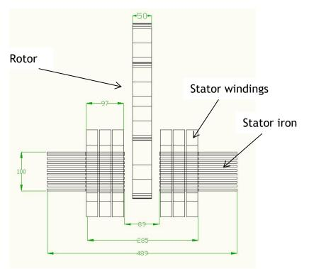
Figure 24. Cross section of rotor inside stator
