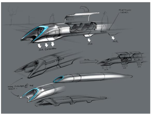
Figure 5. Hyperloop passenger transport capsule conceptual design sketch.
