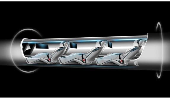
Figure 9. Hyperloop passenger capsule version cutaway with passengers onboard. Hyperloop Passenger Plus Vehicle Capsule
