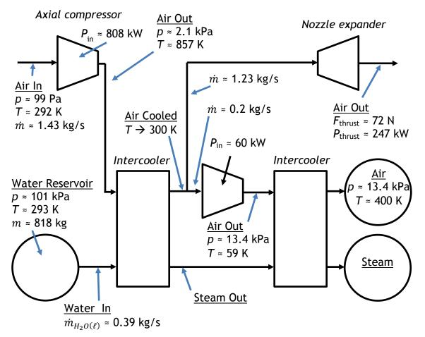
Figure 11. Compressor schematic for passenger plus vehicle capsule.
